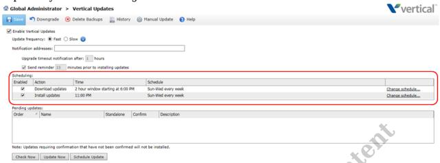
5. The download schedule can be set to any time range that the bandwidth is available. Software will be pulled down and stored on the Wave.
