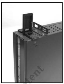
4. The EXU has two alignment pins on the back that will line up with holes on the Wave. Lower the EXU on to the Wave making sure these pins fit into the hole and the backplane connector fits .
